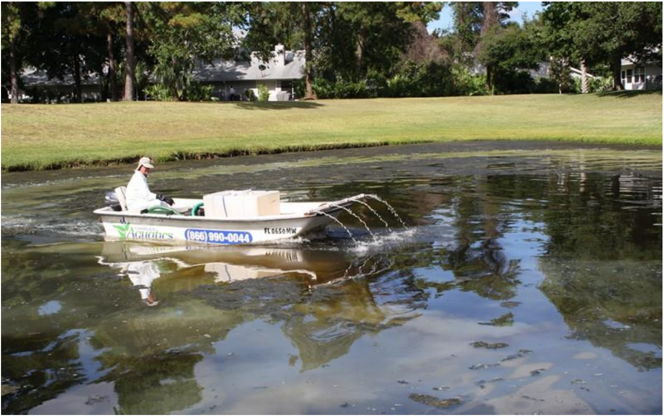
Figure 19. Boat with spray unit, used to spray herbicides.
