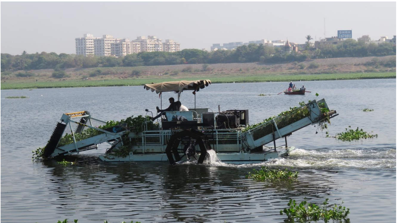
Figure 17. Mechanical removal of water hyacinth by De-weeder/ Weed harvester (SMC).
